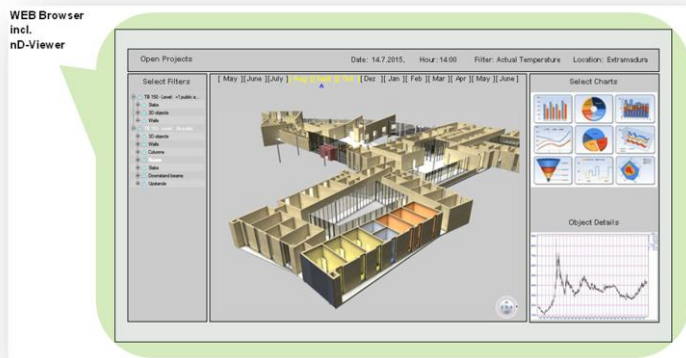
FIGURE: overview of the nD-Navigator components. The access will be realized via Internet. This Graphic User Interface is a first design draft for the nD-Navigator.
